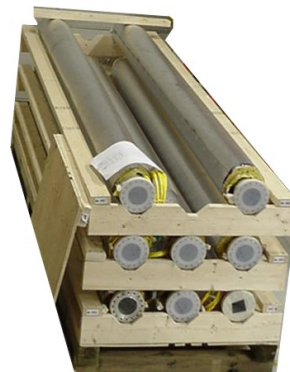
LPCE columns designed and fabricated by Tyne, ready for installation in Texas
