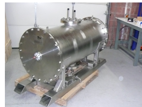
Tritium-compatible electrolyzer modified for service by Tyne
