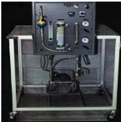
Temporary Mobile Stack monitor
