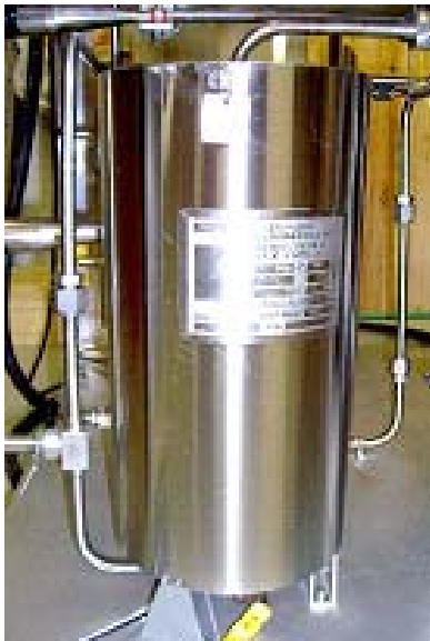
Simple, Single Shell Zirconium Iron Bed
