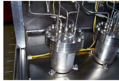
Two 100 Gram Flanged Uranium Beds Installed in a Glove Box
